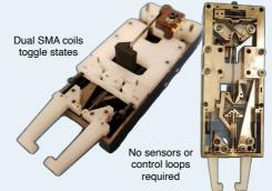
Flexures and buckled beams enable instantaneous motion, solving SMA's biggest weakness: speed
