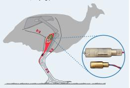
A small implantable device replaces part of the calf muscle to assist movement from inside the leg
