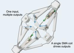
Compliant mechanisms amplify the incredible energy density of smart materials. Grip, return and motion amplification, all through geometry.
